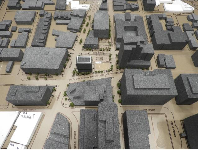
Image 2A: Wind Tunnel Study Model - Existing Configuration
