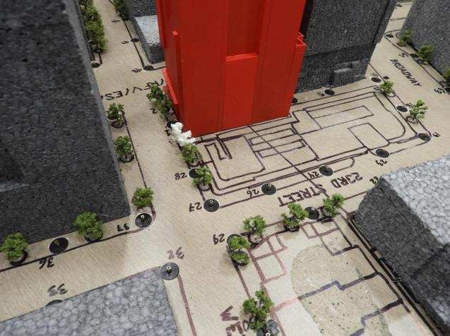
Image 2C: Wind Tunnel Study Model – Existing + Project + Trees Configuration
