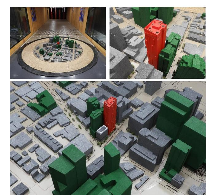
Image 2E: Wind Tunnel Study Model – Project + Cumulative Configuration
