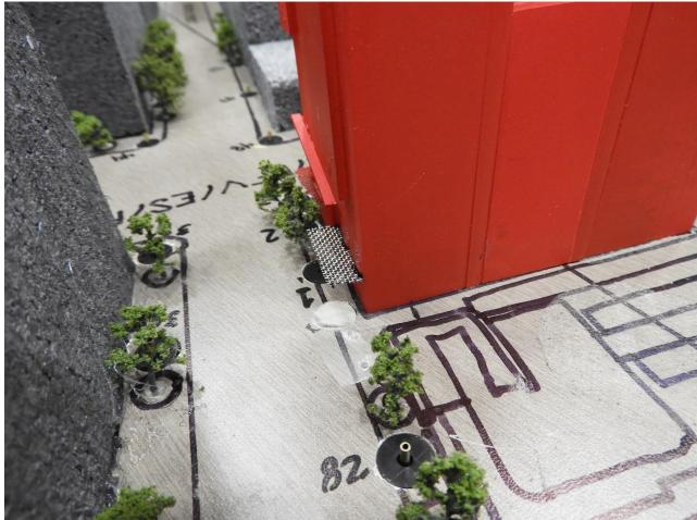
Image 2D: Wind Tunnel Study Model - Existing + Project + Canopy Configuration
