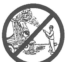
✓ Collect the wash water from washing exposed aggregate concrete and remove it for appropriate disposal off site.
