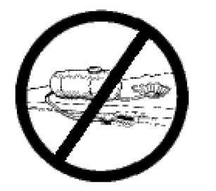
✓ Be sure to notify and obtain approval from the Engineer before discharging water to a street, gutter, or storm drain. Filtration or diversion through a basin, tank, or sediment trap may be required.
