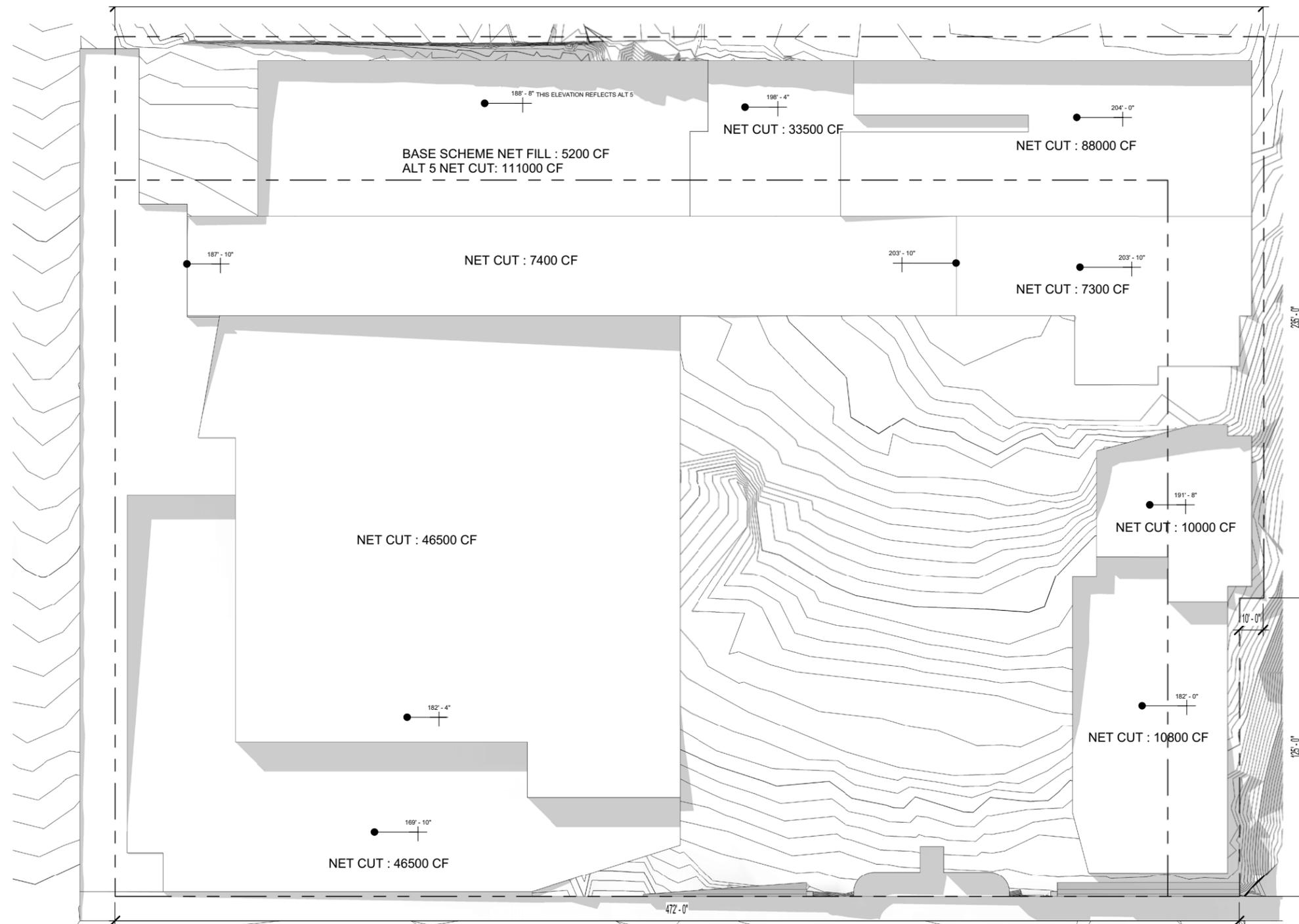
THE CUT & FILL CALCULATIONS ARE PRELIMINARY ESTIMATE. DETAILED CALCULATIONS CAN ONLY BE PERFORMED AFTER DESIGN IS FINALIZED.
