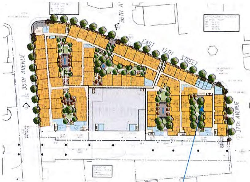
**Revised 2015 FPUD Site Plan for Phase IIA that affect Phase IIB shows** changes in the parking garage affecting both properties. The location of the parking is still along the BART tracks but it is incorporated into the 4-story housing development. Open space is moved to the interior and the future shared 'Paseo' between Phase IIA and Phase IIB is identified. This is an enlargement of half of the original PUD site plan
