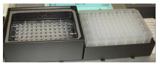
Figure 9-17 Vacuum Wash & Sample Collection Positions
