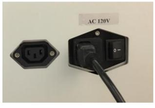
Figure 7-6 VERSA and Vacuum pump Power Connections
