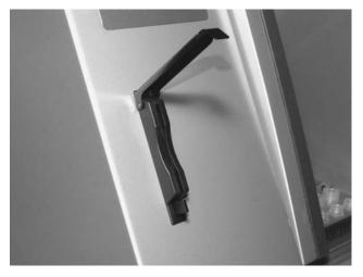
It is extremely important that the EZ1 Card is completely inserted to avoid memory error and loss of essential instrument data.
