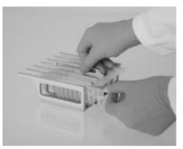
Figure 3. Ease of setup using reagent cartridges. A sealed, prefilled reagent cartridge. Fill levels vary, depending on the type of reagent cartridge. I Loading reagent cartridges into the cartridge rack. The cartridge rack itself is labeled with an arrow to indicate the direction in which reagent cartridges must be loaded.
