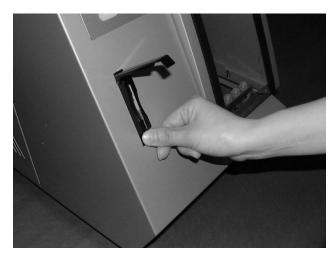
3. Press the button at the bottom of the EZ1 Card slot.
