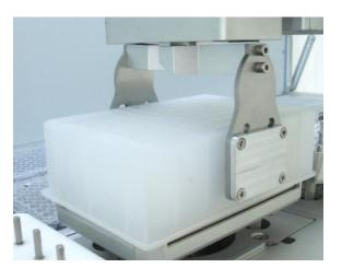
Figure 9-63 Gripper Holding Deep Well Plate
