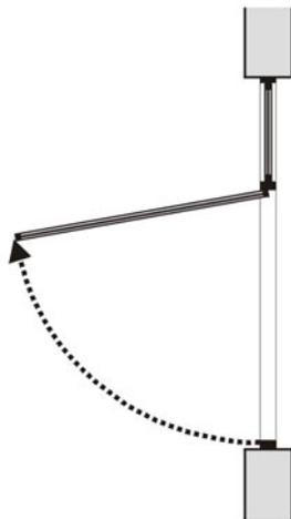
2.2.4c Openable awning windows should open inward so that they do not interfere with the sidewalk.
