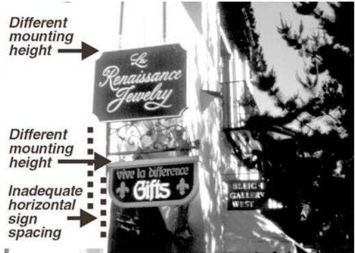
1.3.5 Avoid placing projecting signs at different heights and closer together than 40 feet
